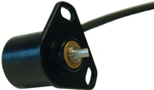
The output of a rotary hall sensor is a voltage which changes in direct proportion to the shaft angle. A constant voltage is required across the supply and ground wires of the sensor. No internal end stops are fitted, so continuous rotation is possible. The sensor consists of a Hall Effect element, a shaft and a magnet. When the angular position of the sensor changes relative to the magnet, the change in magnetic field in the sensor results in a change in output voltage.
